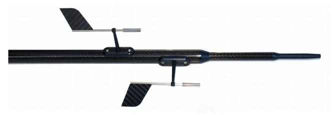
The FTB-1 air data boom can be used with the extended ADC-10X air data computer. The ADC-10X is based on the well known ADC-10 but enhanced with two inputs for the vanes. The extended ADC outputs additional AoA and AoS data labels over the RS-485 data interface. The data labels are calibrated and aerodynamically corrected for zero-point and non-linearity.
