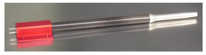
The mount features Simtec's PSS-8 probe on a strong and light carbon fiber tube. The probe is made of strong aircraft grade aluminum for maximum rigidity. The static ports are drilled into to aluminum part of the probe for highest precision and quality. The mount can be attached on the UAV using two or four M4 screws. To keep the pressure lag of the system to a minimum and balanced between total (Pt) and static pressure (Ps) the internal volume of the system is kept as low as possible.
